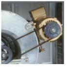
Adjustable motor mounts provide easy alignment and belt tensioning
